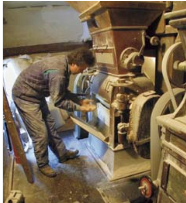
The old Felix Mill was built in the early 1920s and it is still in a perfect working condition. It is an old rolling mill that is mostly hand made of wood. The mill has only one turbine and many belts that transmit the driving power throughout the mill.
